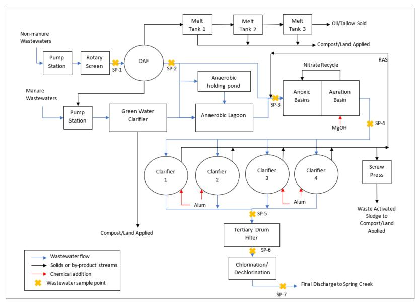
Figure 1. SBC-Hyrum Wastewater Treatment System
